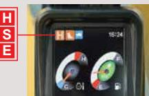
**H-mode:** For heavy duty operation, when a higher performance level is required.
